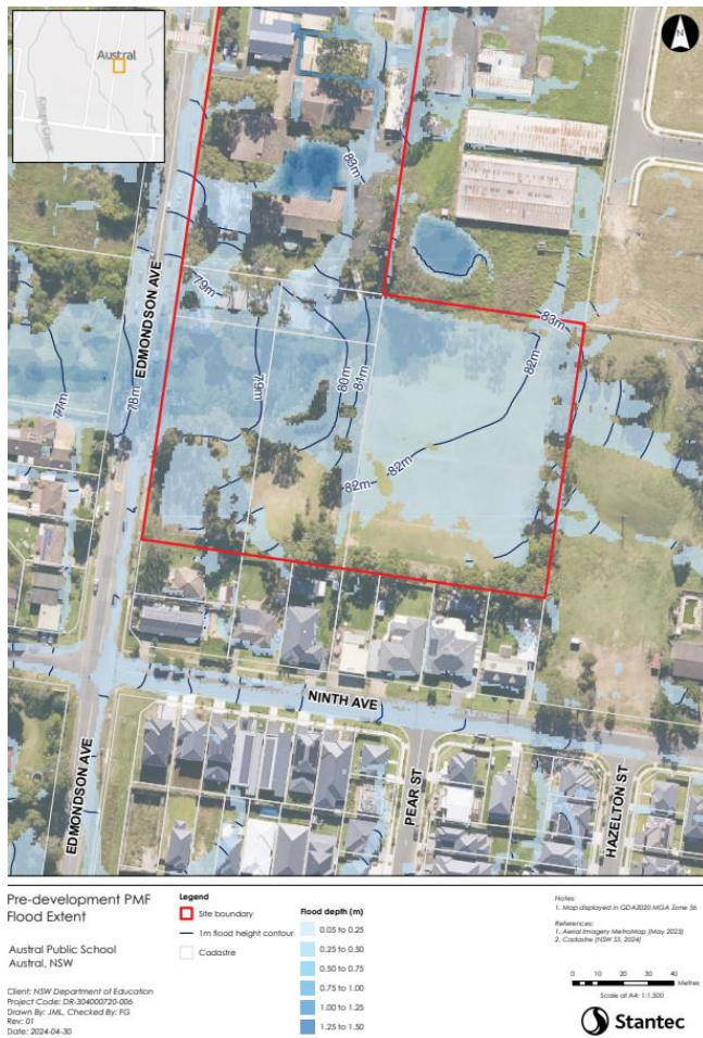
Figure 61: Pre-development PMF flood extent (Source: Stantec)
